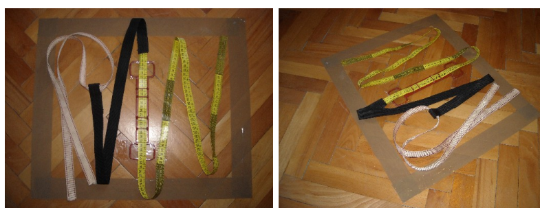
Figure 1. A device for measuring height of vertical jump (Abalak's method).
